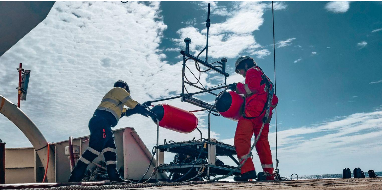
Geo Marine operators deploying a stacked sparker
