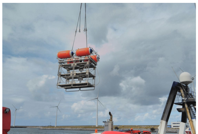
Geo-Source Triple 800 sparker sources being loaded onto the vessel
