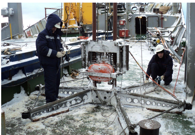
Operators performing vibro-core operations
